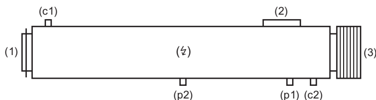
Figure 2 : Configuration with ERD (3) mounted at the front end of the test vessel
