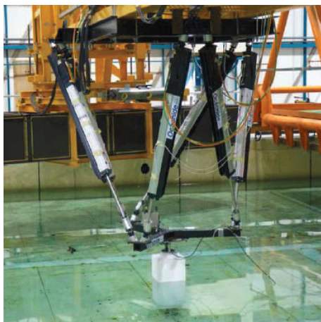
Figure 131: Use of hexapod system. Left – forced motion in water, Right – sloshing model tests.
