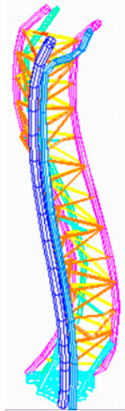
Figure 8 : Modal analysis of the pump mast
